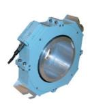
The Series 420 Shaft Power Meter System provides a display of the shaft torque, rotary speed and power. The torque signal is derived from strain gauges installed on to the shafts. The shaft speed signal is derived from an on-shaft speed pick off within the stator unit. These signals are transmitted from the shaft rotor to the shaft stator unit. These signals are then transmitted to the Control Unit and calibrated to provide a display of torque, speed and power for either a single or dual shaft.
